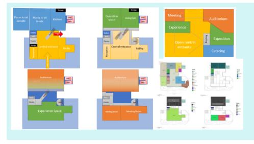
The floor plan has been filled with the functions that has to fit into the building. In this stage the routing has been taken into account. The floor plan has also been worked out to a definitive version which is in miniature presented in the right corner.
